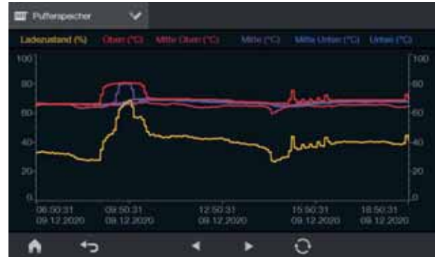
The system characteristics can be tracked over a period of up to 4 weeks directly on the system controller. With the aid of these values, the energy system can be optimised and its efficiency and cost effectiveness enhanced.
